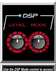
Use the DSP Mode control to access any of the 16 built-in digital effects. Use the Level control to mix in the desired amount of each effect.
